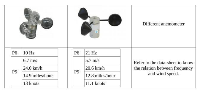
If you want to reed Hz on the display, use P5=1 and P6=1. If you want to read RPM use P5=60, P6= the number of pulses in one rotation.
